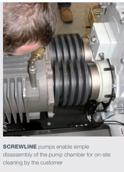
**SCREWLINE** pumps enable simple disassembly of the pump chamber for on-site cleaning by the customer
